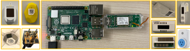
Figure 7: Gateways and devices in our deployment. Column-wise, top to bottom: CO 2 sensor, Occupancy sensor, Estimote beacon, Power meter, Raspberry Pi, Light sensor, Temperature sensor, Location beacon, Contact sensor, Smart socket.
